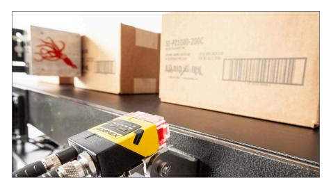
SquidCheck is integrated with a Cognex® reader and Squid Ink printer to ensure that codes are present, scannable, and accurate.
