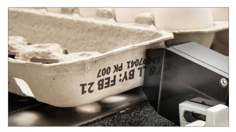
**1)** CoPilot Flex's compact printhead is designed to match the slope of the egg carton, resulting in highquality print.
